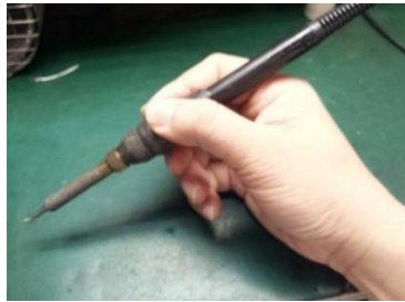
Gambar 8.8 Cara memegang solder
