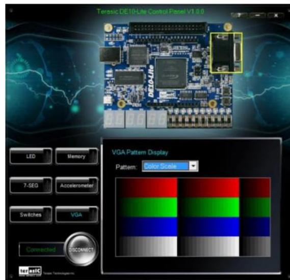
*gambar 1.1.4.5 controlling VGA display under control panel*
