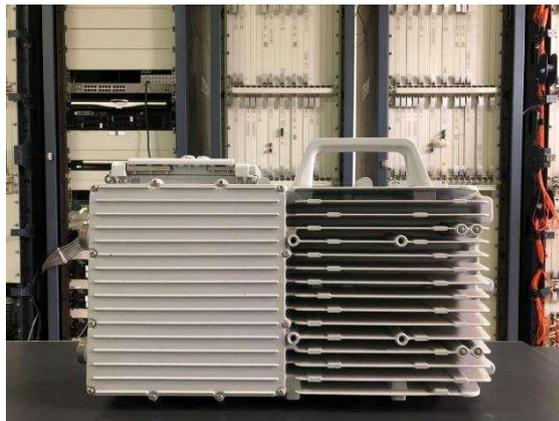
Gambar 1.4 *Remote Radio Unit (RRU)*
